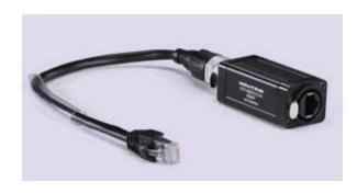
Neutrik® Ethercon® cables last far longer than standard RJ-45 cables because the contacts are protected by a heavy duty aluminum shroud. But the shroud prevents the cables from connecting to standard RJ-45 jacks. The Ethercon® to RJ-45 Adapter allows Neutrik® Ethercon® cables to be plugged into standard RJ-45 jacks
