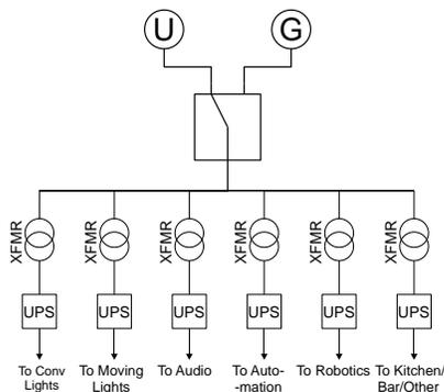
Fig. 1. Simplified 1 line diagram of input power to facility. Overcurrent devices not shown.
